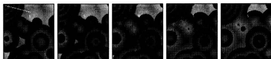
3a Sequential images of BZ reaction (λ = 500 nm) Time interval = 5s, Color image 32.0 mm square
